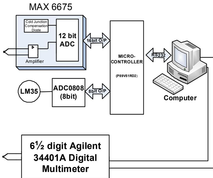
Fig. 5: Calibration System
