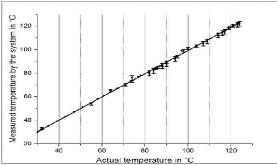
Fig. 6: Calibration Curve
