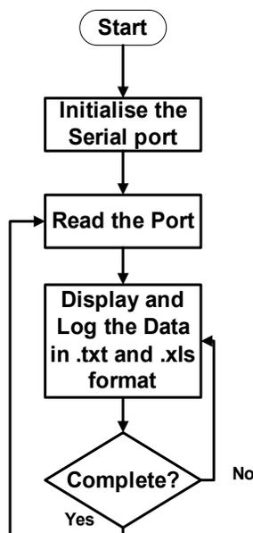
Fig. 4: Flowchart of the Software
