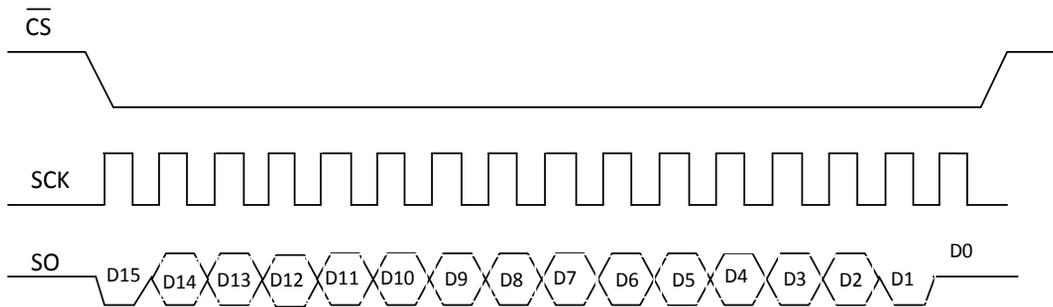
Figure 2: Data framing of 16-bit output data of MAX6675 (datasheet of MAX6675)
