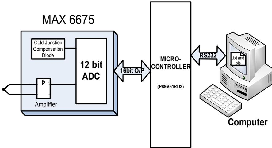
Fig. 1: Block diagram of the temperature measurement system
