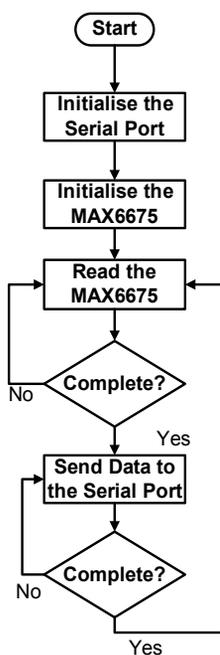
Fig. 3: Flowchart of the Firmware
